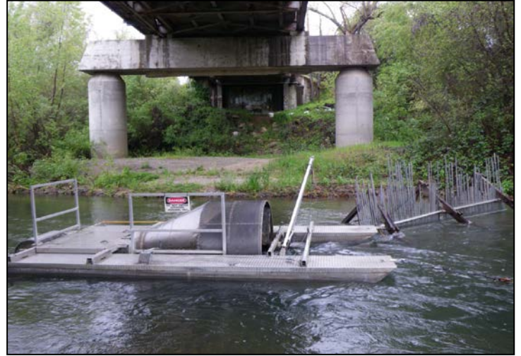
Pictured at left is a downstream migrant trap on Mill Creek. At right is a downstream migrant trap on Dry Creek.
