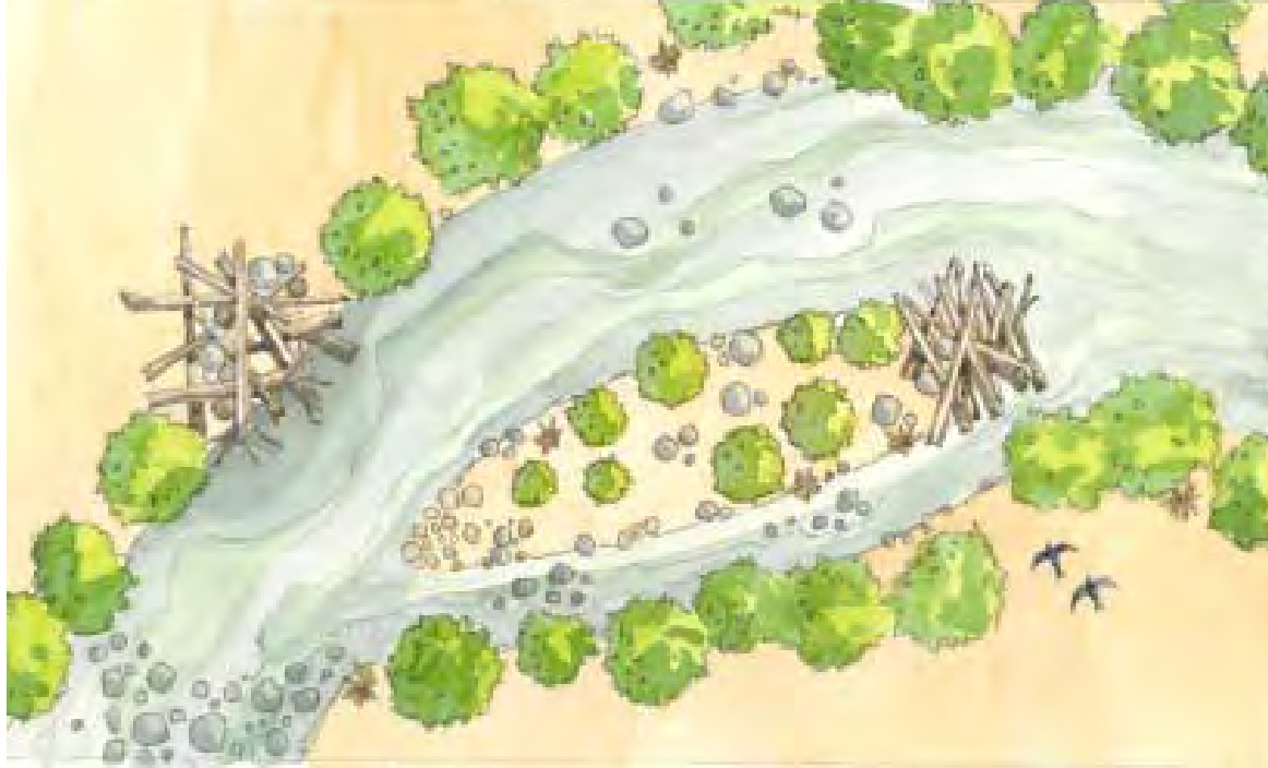
Figure 5. Conceptual depiction of side channel.
