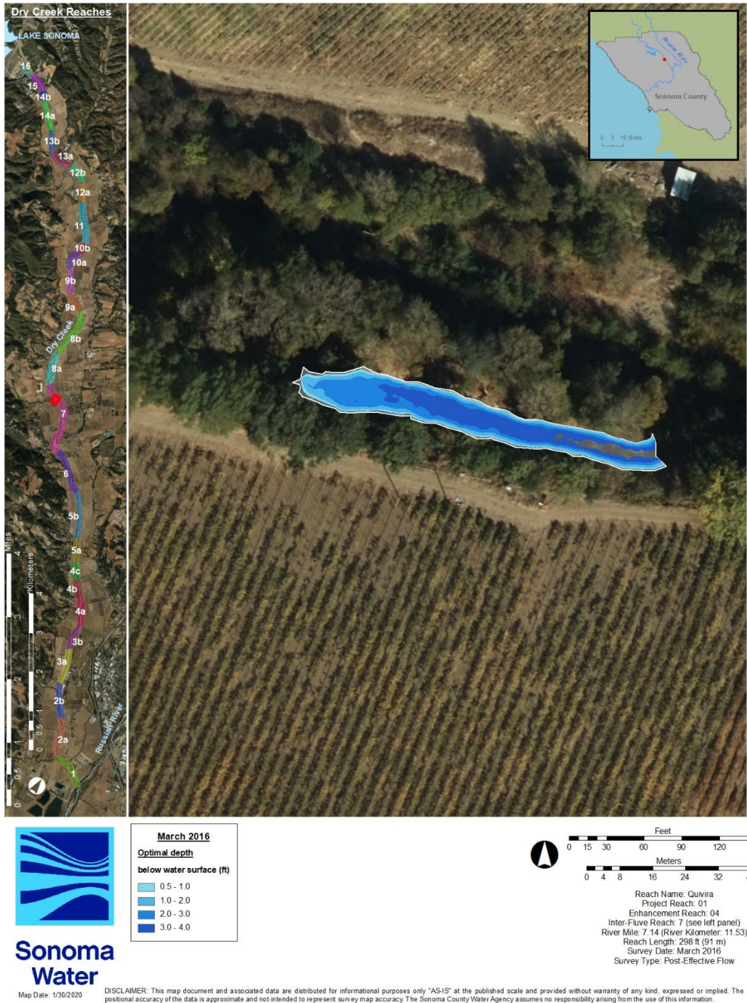
Figure QU-2. Optimal water depth for fry (0.5-2.0 ft) and parr (2.0-4.0 ft) within the Quivira enhancement reach, March 2016.
