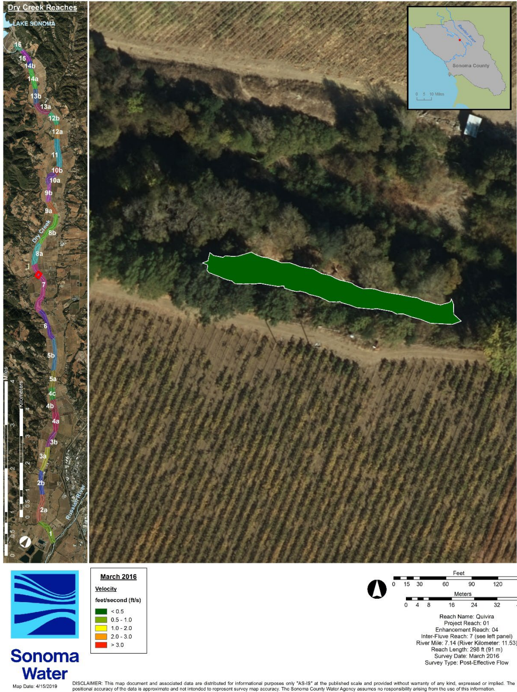
Figure QU-3. Measured water velocity within the Quivira enhancement reach, March 2016.
