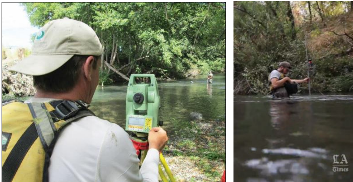
Figure 5.2. 1. Dry Creek effectiveness monitoring. At each data point, we collected geographic location (latitude, longitude, elevation), and water depth and velocity by aiming the total station at a USGS topset rod fit with a survey prism and a flow meter.
