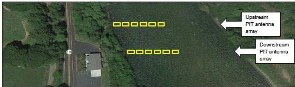
Figure 4.5.2. Flat plate antenna arrays at Duncans Mills (rkm 10.44 and 10.46). Rectangles represent individual flat plate antennas.
