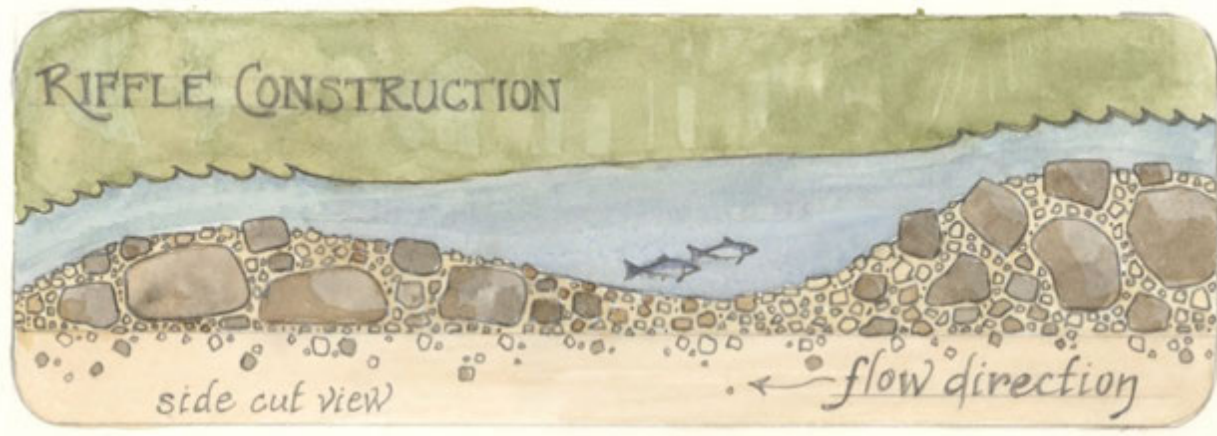
Figure 7. Conceptual depiction of riffle construction.
