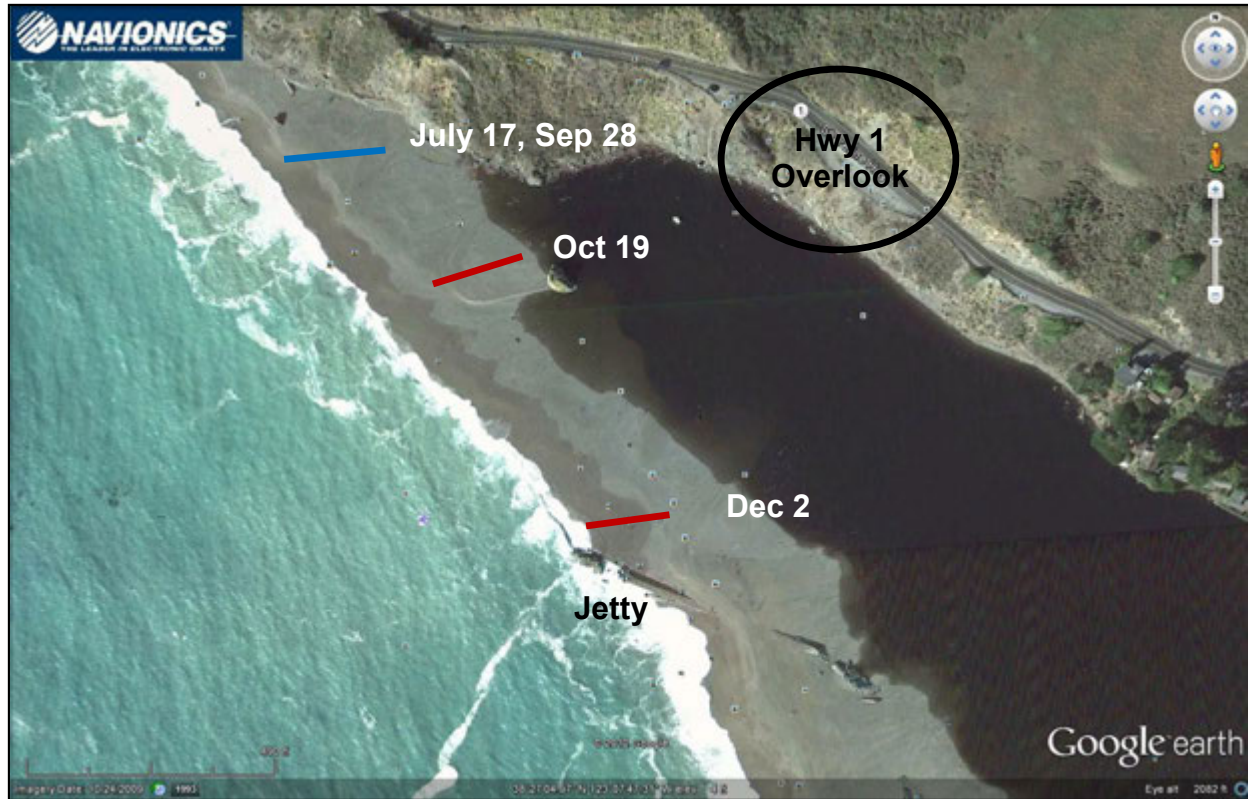
Figure 4.6. Locations of beach management activities in 2017 at the Russian River mouth, Goat Rock State Beach. Lines crossing the barrier beach are pilot channels for artificial breaching (red) and outlet channels to form a lagoon (blue). Self-breach events are not shown.
