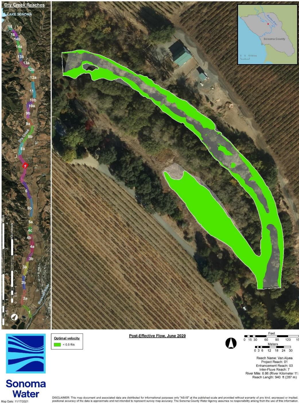
Figure 49. Optimal water velocity for fry and parr (< 0.5 ft/s) within the Van Alyea enhancement reach, June 2020.
