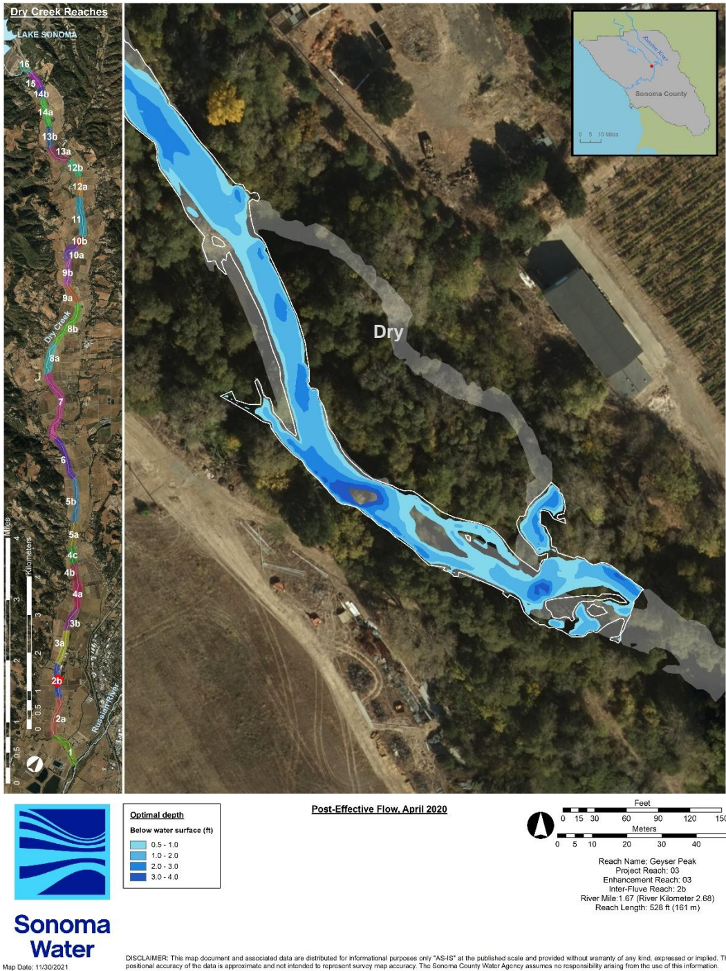
Figure 83. Optimal water depth for fry (0.5-2.0 ft) and parr (2.0-4.0 ft) within the Geyser Peak enhancement reach, April 2020.
