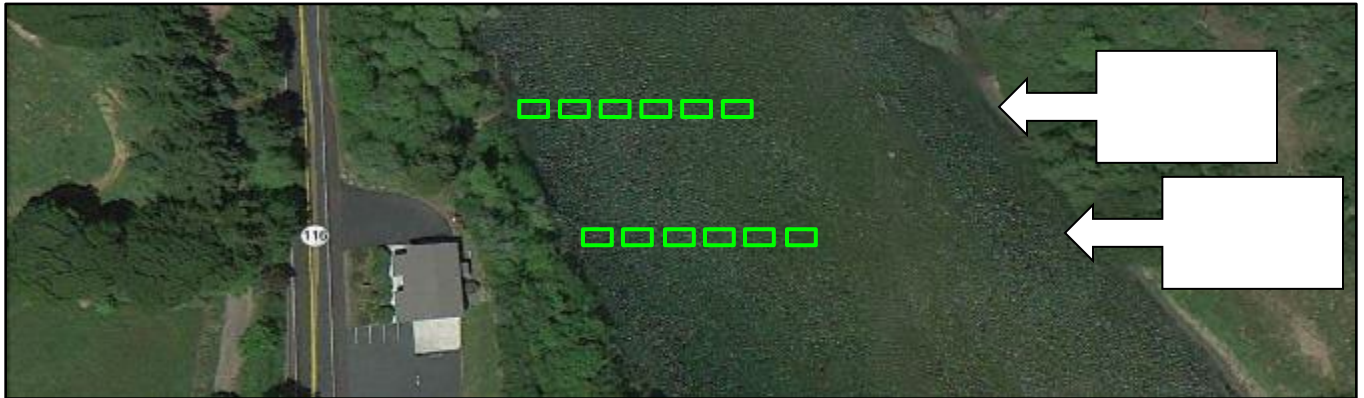
Figure 4.5.2. Flat plate antenna arrays at Duncans Mills (river km 10.44 and 10.46). Rectangles represent individual flat plate antennas.
