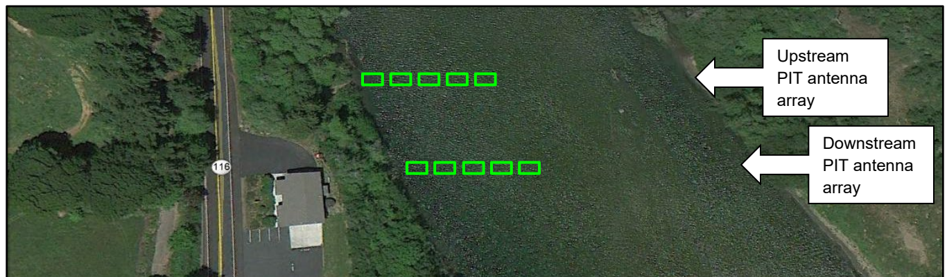
Figure 4.5.2. Flat plate antenna arrays at Duncans Mills (river km 10.46). Rectangles represent individual flat plate antennas.
