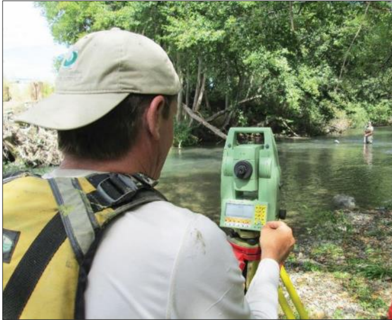
Figure 5.2.1. Dry Creek effectiveness monitoring. At each data point, we collected geographic location (latitude, longitude, elevation), and water depth and velocity by aiming the total station at a USGS topset rod fit with a survey prism and a flow meter
