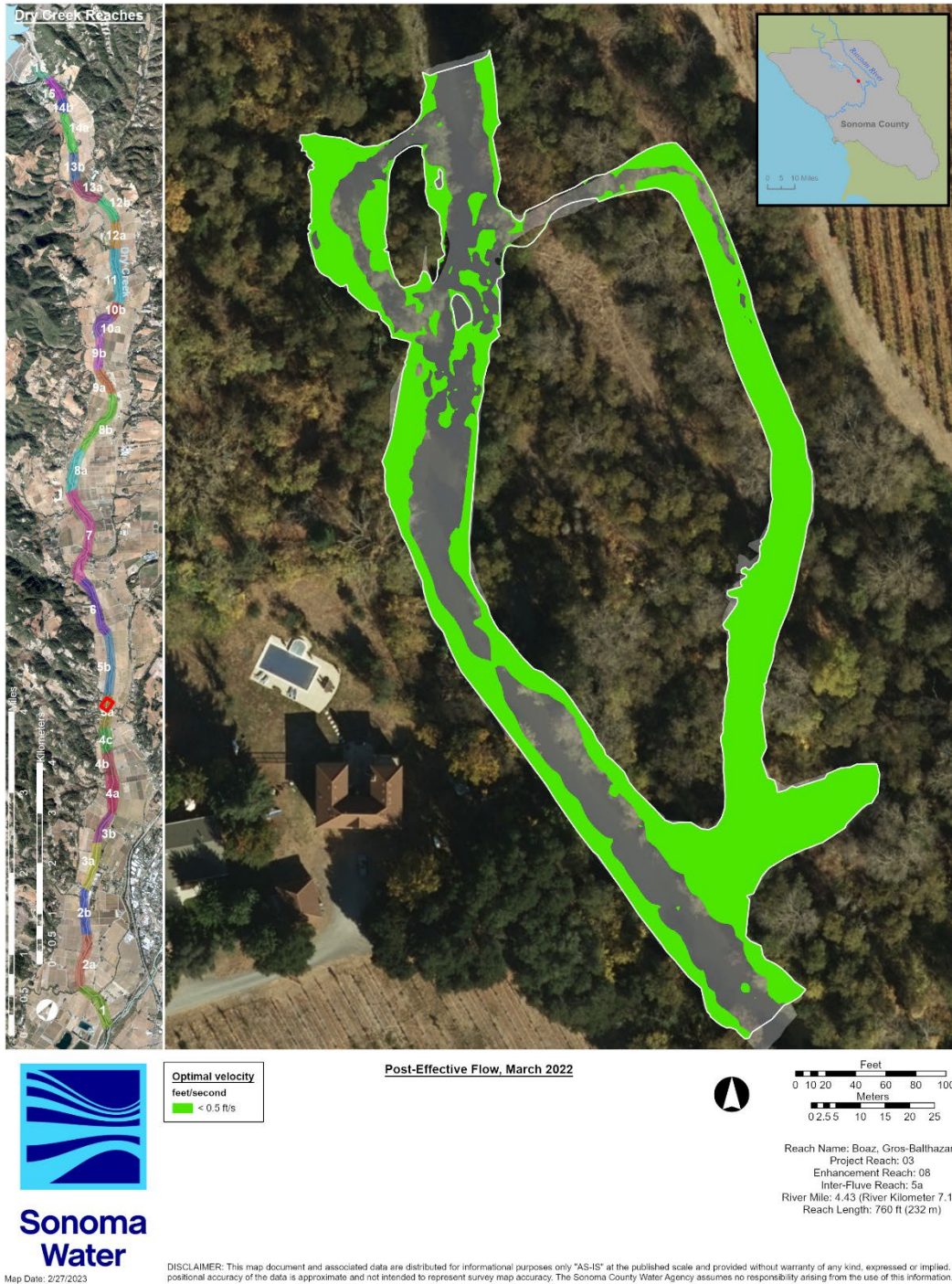
Figure 84. Optimal water velocity for fry and parr (< 0.5 ft/s) within the Boaz Gros-Balthazard enhancement reach, March 2022.
