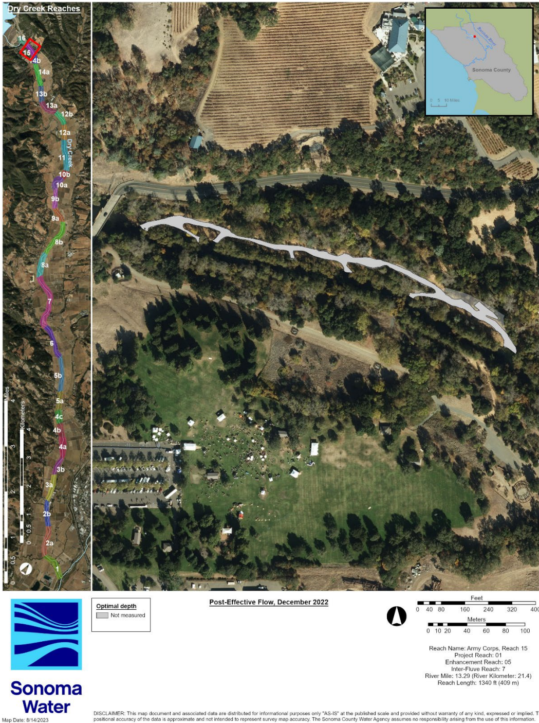
Figure 34. Optimal water depth for fry (0.5-2.0 ft) and parr (2.0-4.0 ft) within the Army Corps enhancement reach, December 2022.
