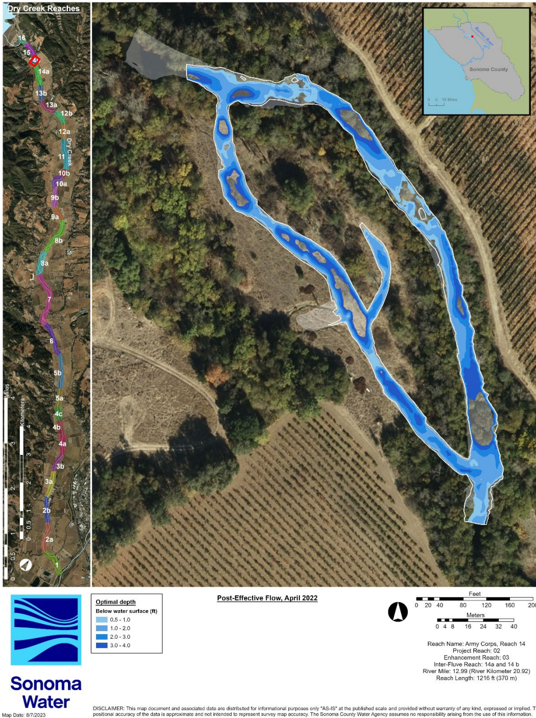
Figure 46. Optimal water depth for fry (0.5-2.0 ft) and parr (2.0-4.0 ft) within the Army Corps Reach 14 enhancement reach, April 2022.
