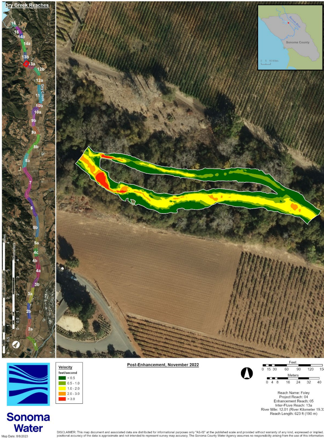
Figure 23. Measured water velocity within the Foley enhancement reach, November 2022.
