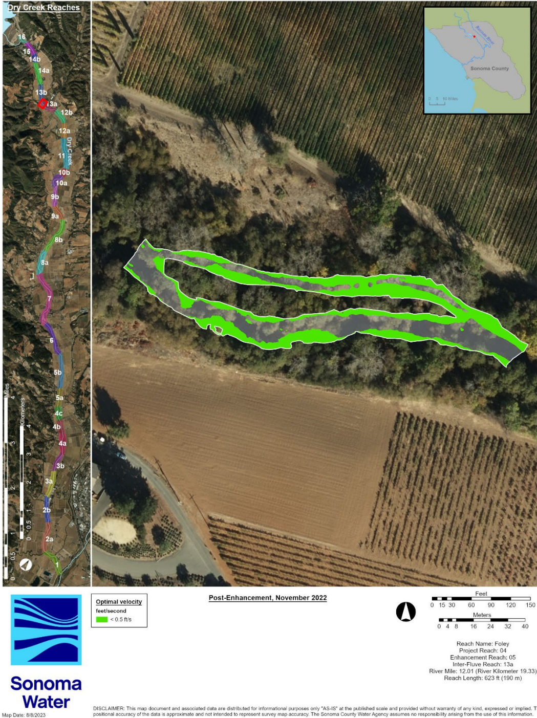
Figure 24. Optimal water velocity for fry and parr (< 0.5 ft/s) within the Foley enhancement reach, November 2022.
