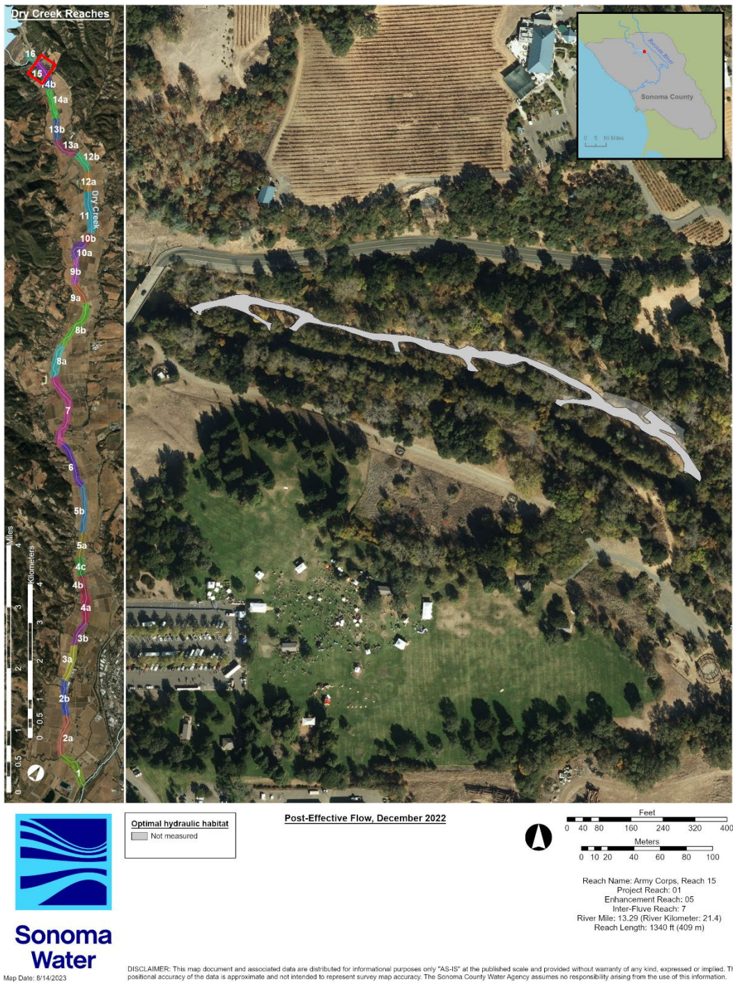
Figure 37. Optimal hydraulic habitat for fry (<0.5 ft/s, 0.5-2.0 ft) and parr (<0.5 ft/s, 2.0-4.0 ft) within the Army Corps enhancement reach, December 2022.
