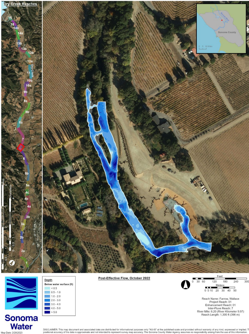
Figure 69. Measured water depth within the Farrow Wallace enhancement reach, October 2022.
