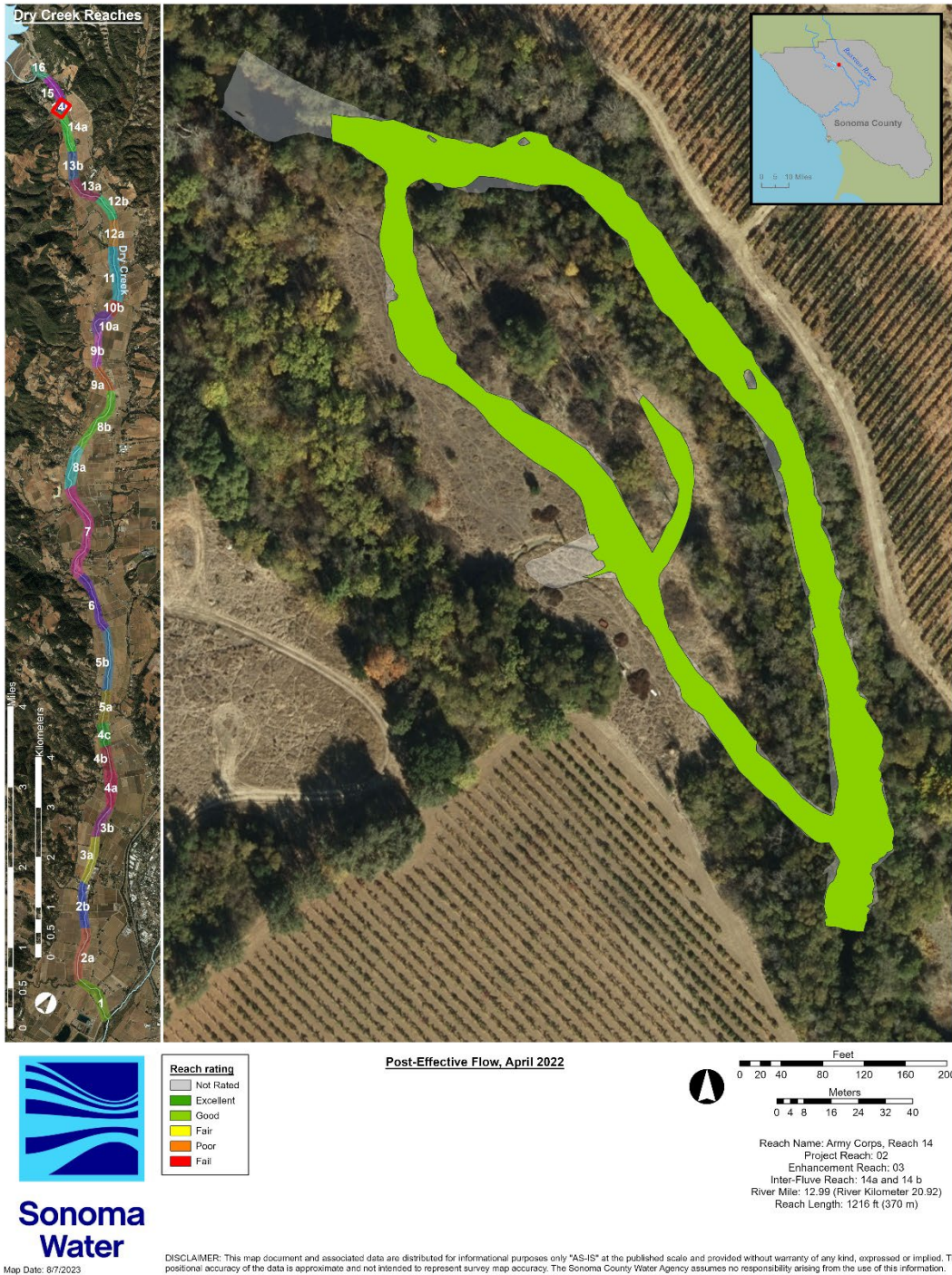
Figure 56. Post-effective flow reach rating for the Army Corps Reach 14 enhancement reach, April 2022.
