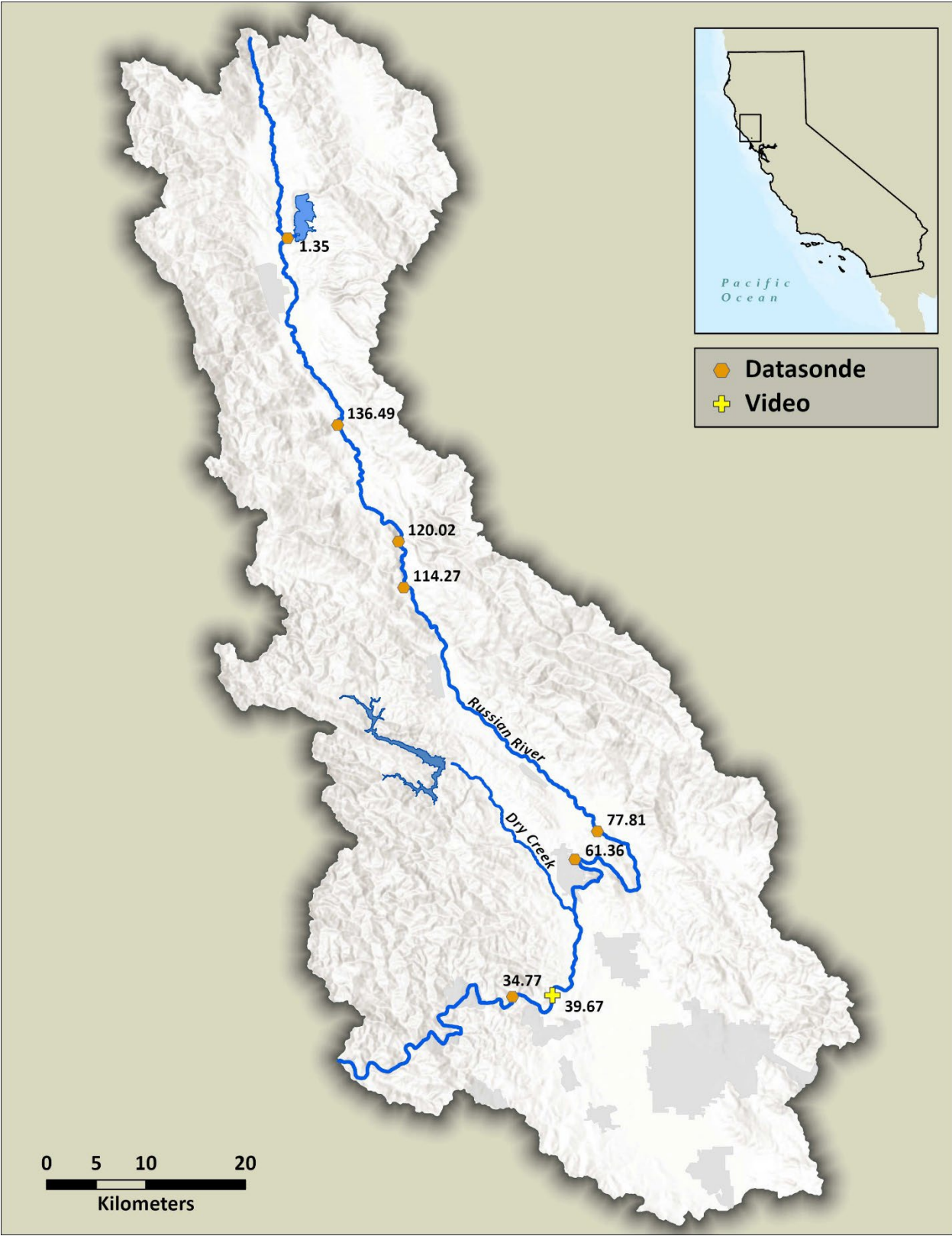
Figure 4-1. The river Km for sites on the Russian River where continuous temperature and dissolved oxygen data was collected by USGS or Sonoma Water in 2022 and used in this report.
