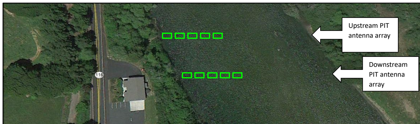
Figure 4.5.2. Flat plate antenna arrays at Duncans Mills (river km 10.46). Rectangles represent individual flat plate antennas.
