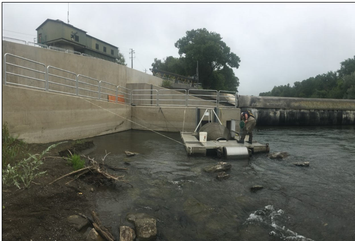
Figure II-2. Downstream migrant trap at Sonoma Water's Mirabel dam in Forestville (Chinook smolt LCM station, rkm 39.67).
