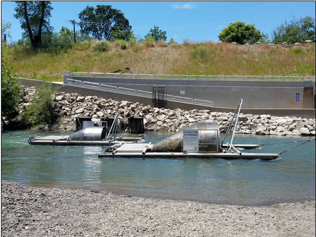
Figure 3. Downstream migrant traps at Sonoma Water’s Mirabel dam in Forestville (Chinook smolt LCM station, rkm 39.67).
