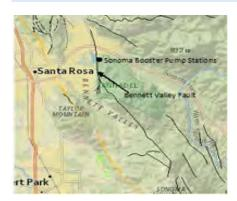
Implement measures to increase water supply reliability and mitigate the risk of pipeline rupture in the vicinity where the 20 inch diameter Sonoma Aqueduct and 24 inch diameter Oakmont Pipeline traverse the Bennett Valley Fault system in Rincon Valley. Construction implementation is reliant in part on securing grant funding.
