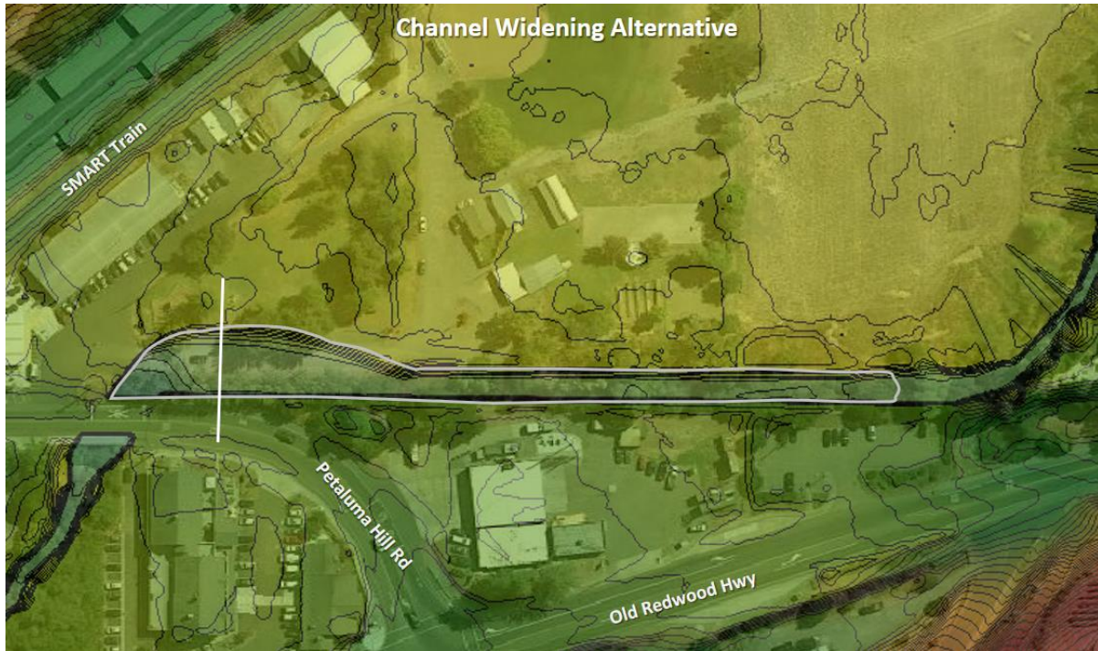
Figure 20. Bank Widening Alternative. Grey outlines indicate extent of channel widening. White line shows location of cross section in Figure 21.
