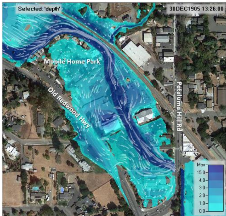
Figure 15. Existing condition predicted flood depths and extent during the 10-yr storm peak in downtown Penngrove.
