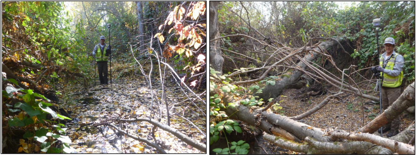
Figure 2. Photos of surveyed riffle crest (top left), log jam causing elevated hydraulic roughness (top right).
