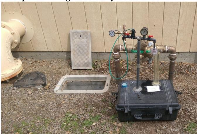
**Set-up for testing water quality**
