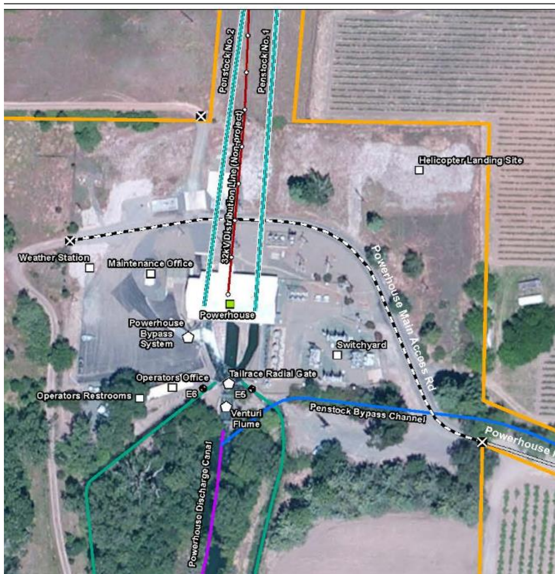
Figure 2-6. Schematic of Potter Valley Powerhouse and flow measurement locations E5 and E6 (adapted from PG&E 2017).
