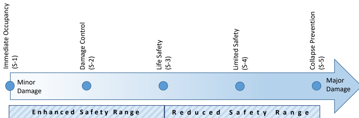
Figure 6: ASCE 41-17 Structural Performance Levels – (Source: ASCE/SEI 41-17: Performance Objectives and Seismic Hazard Changes – February 2019)
